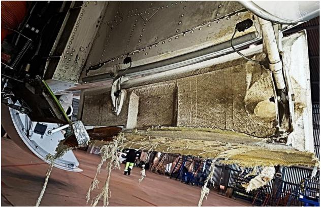
Picture 24 View of NLG front doors damage from inside NLG compartment
