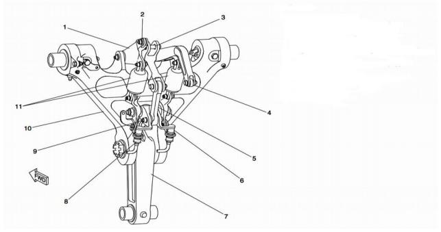
The drag strut assembly stabilizes the shock strut in either the retracted or the extended position. The drag strut assembly has the components that follow:
