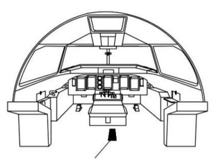
floor of the flight compartment under the LANDING GEAR ALTERNATE EXTENSION door.
