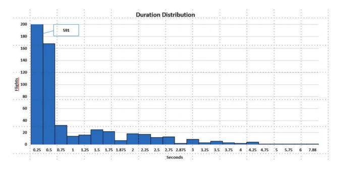
On YL-BAI maximum duration from Nose WOW sensor activation to Main WOW sensor activation was 3.75 seconds with corresponding 1.15G landing acceleration value (October 2015).
