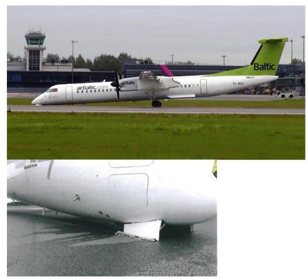
**Picture 16 and 16A** After the aircraft had come to a complete stop on the runway the NLG appeared to have fully collapsed, which resulted in NLG front door damage.
