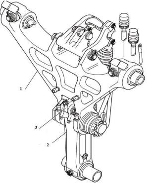
The lower lock link (3) is installed on the lower drag strut (2) and is connected to the upper lock link. The upper lock link is installed on the upper drag strut and is connected to the lock link assembly. The over centering action of the upper and lower lock links makes a mechanical lock when the gear is in the retracted and the extended positions.
