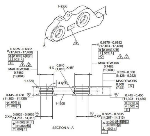
Picture 79 Drag Strut Assembly bushing (1320)
