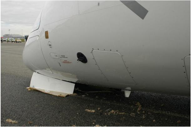
Picture22 NLG front doors damage
