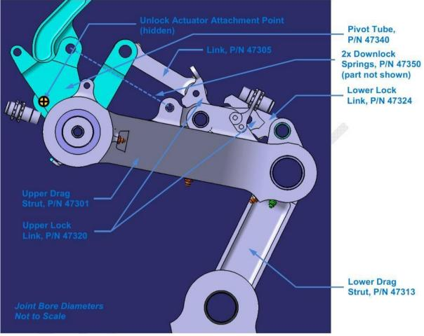
Picture 76 Q400 Nose Landing Gear Drag Strut Assembly
