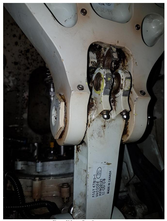
**Picture 28 Lower Drag Strut** After removing from aircraft it was stated that the lugs of the Lower Drug Strut for the Lower Lock Link was damaged.
