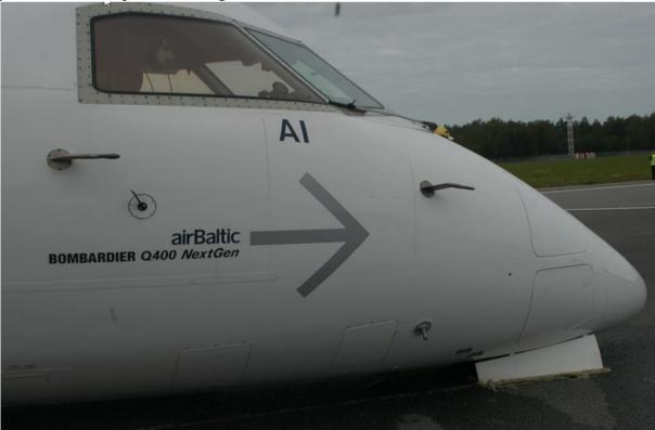
Picture 21 NLG front doors damage
