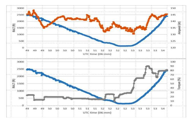
Low pass at minimum 126FT Radio altitude flown. Airspeed and torque values for time period 06:49 - 06:54 UTC displayed.
