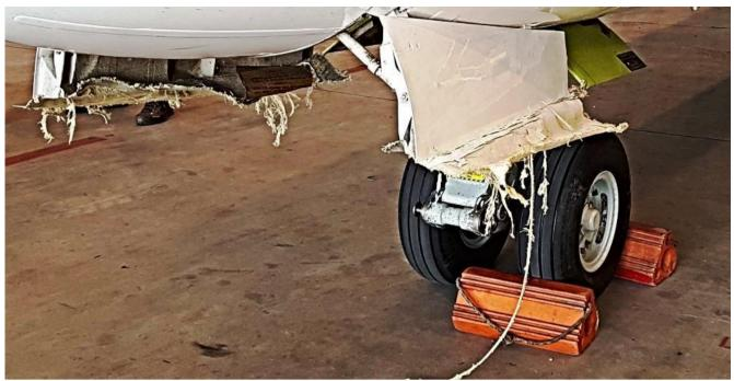
Picture 17 Damages of NLG front doors
