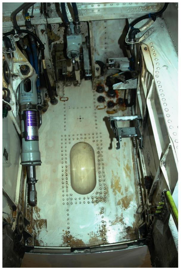
Picture 30 NLG compartment after components removing.
