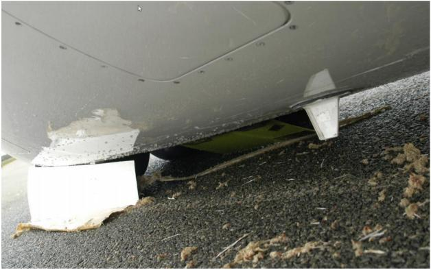
Picture 25 NLG front doors damage
