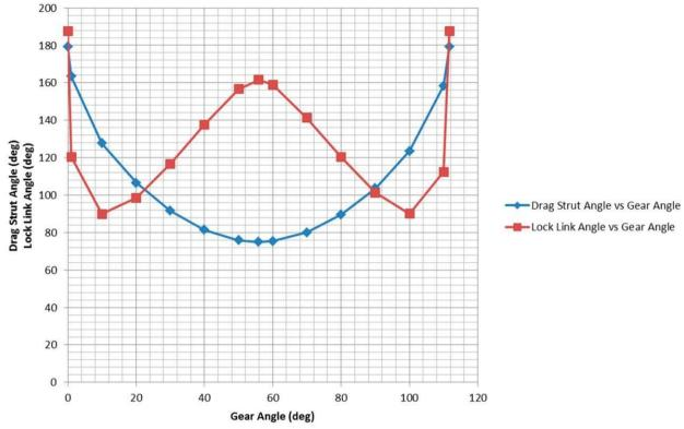
Picture 77 Drag Strut Angle and Lock Link Angle vs Gear Angle
