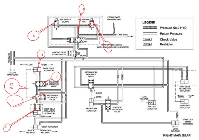
Figure 3 Gear Up and Locked Doors Closed
