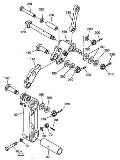
**Picture 25 NLG Drag Strut Assembly, Ilustrated Parts Catalog (IPC)** During the first inspection was found that nut 210 of pin 170 of upper lock drag strut and part of pin was detached. NLG Drag Strut Assembly was removed from aircraft for inspection.
