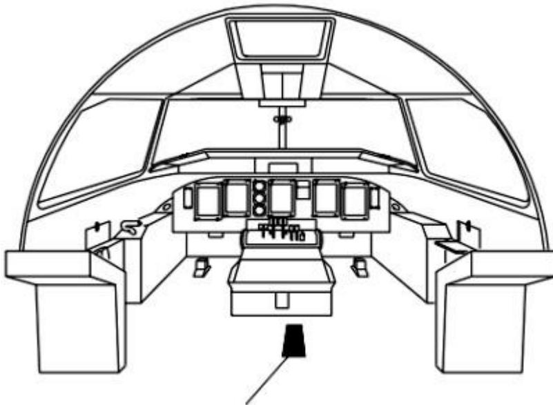
**NLG alternate release locator**
