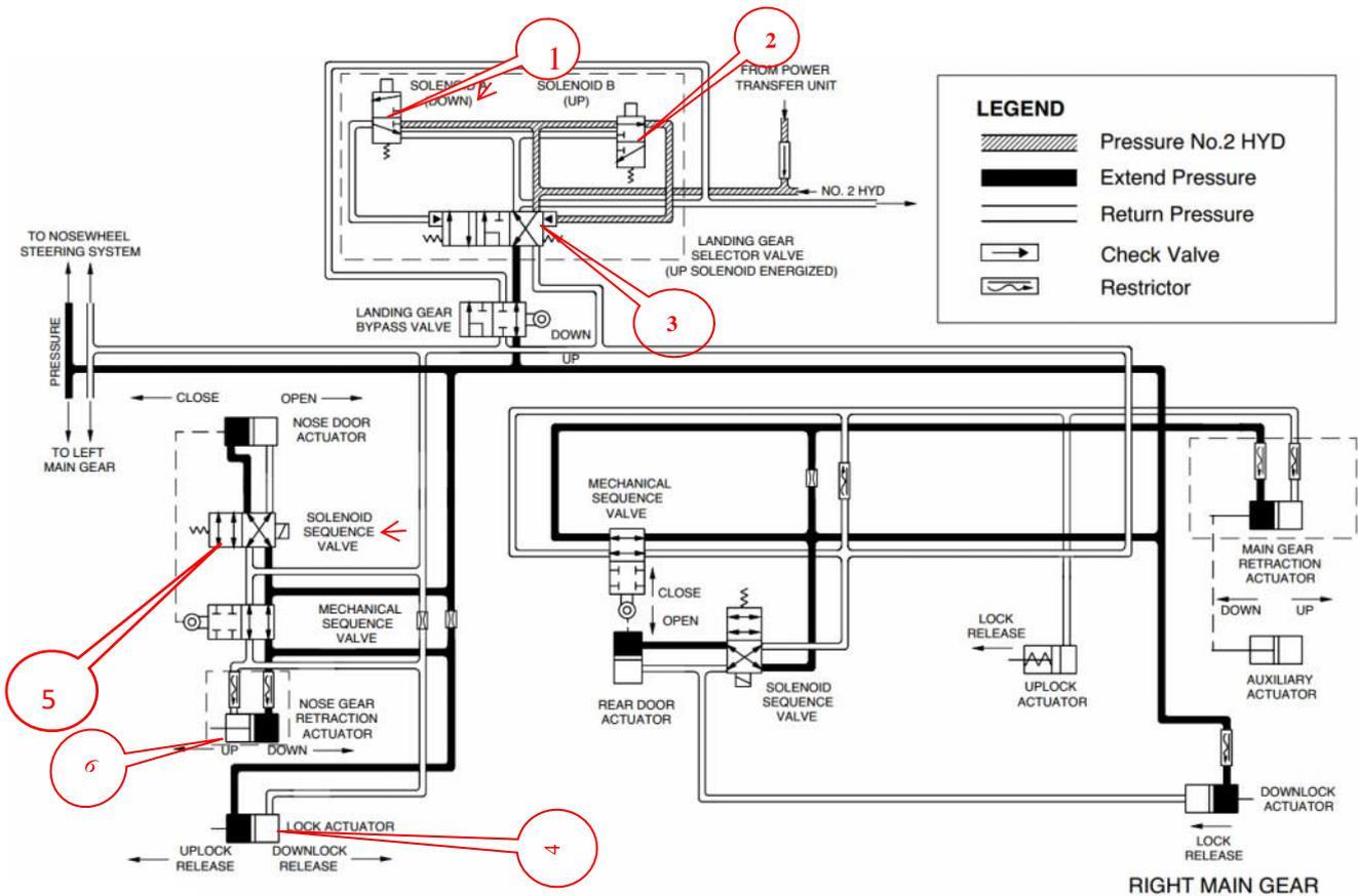
**Figure 2 Initial Up Selection Doors Open (before reaching the fully UP position)**
