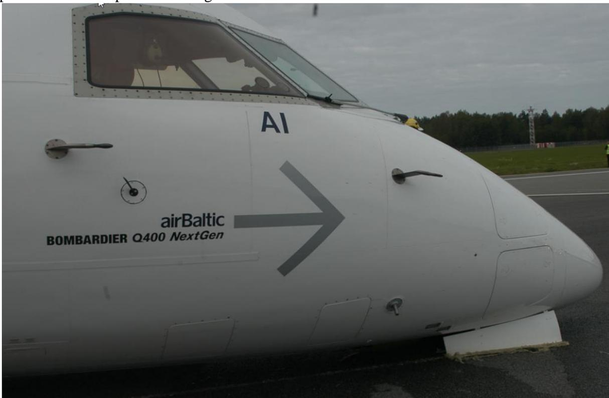
**Picture 21 NLG front doors damage**
