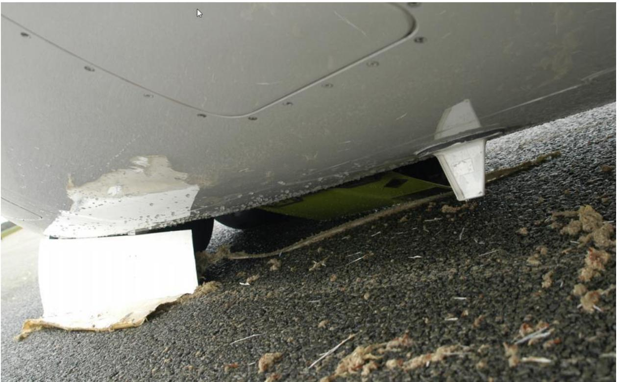
**Picture 25 NLG front doors damage**
