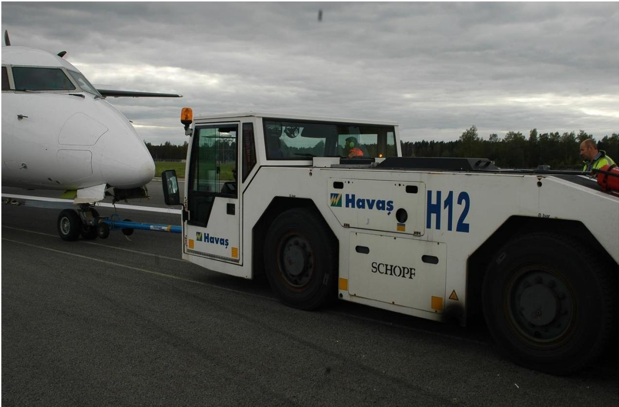
**Picture 28 Removing aircraft from RWY procedure**
