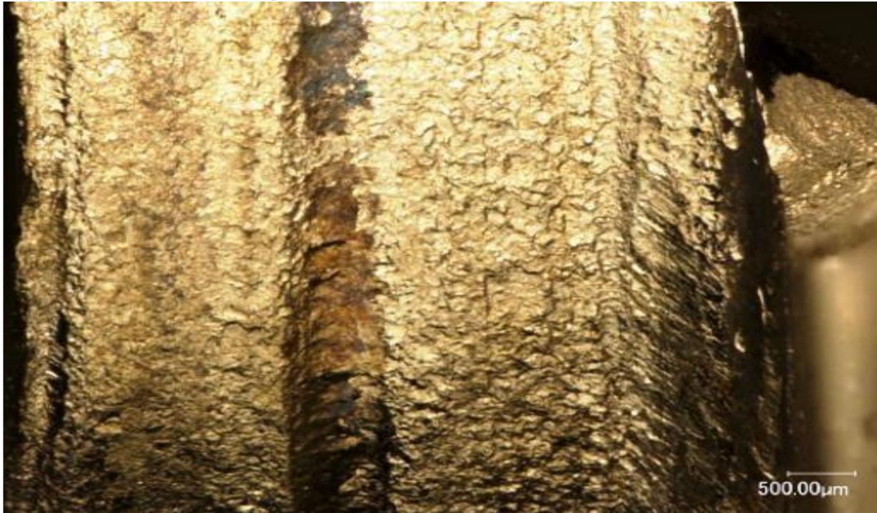
**Picture 81 Optical microscopy image of the mating surface of the bushing with the inside of the LLL pin hole**
