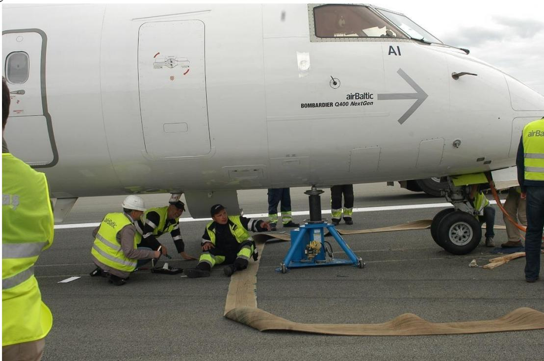
**Picture 26 Preparation of aircraft lifting**
