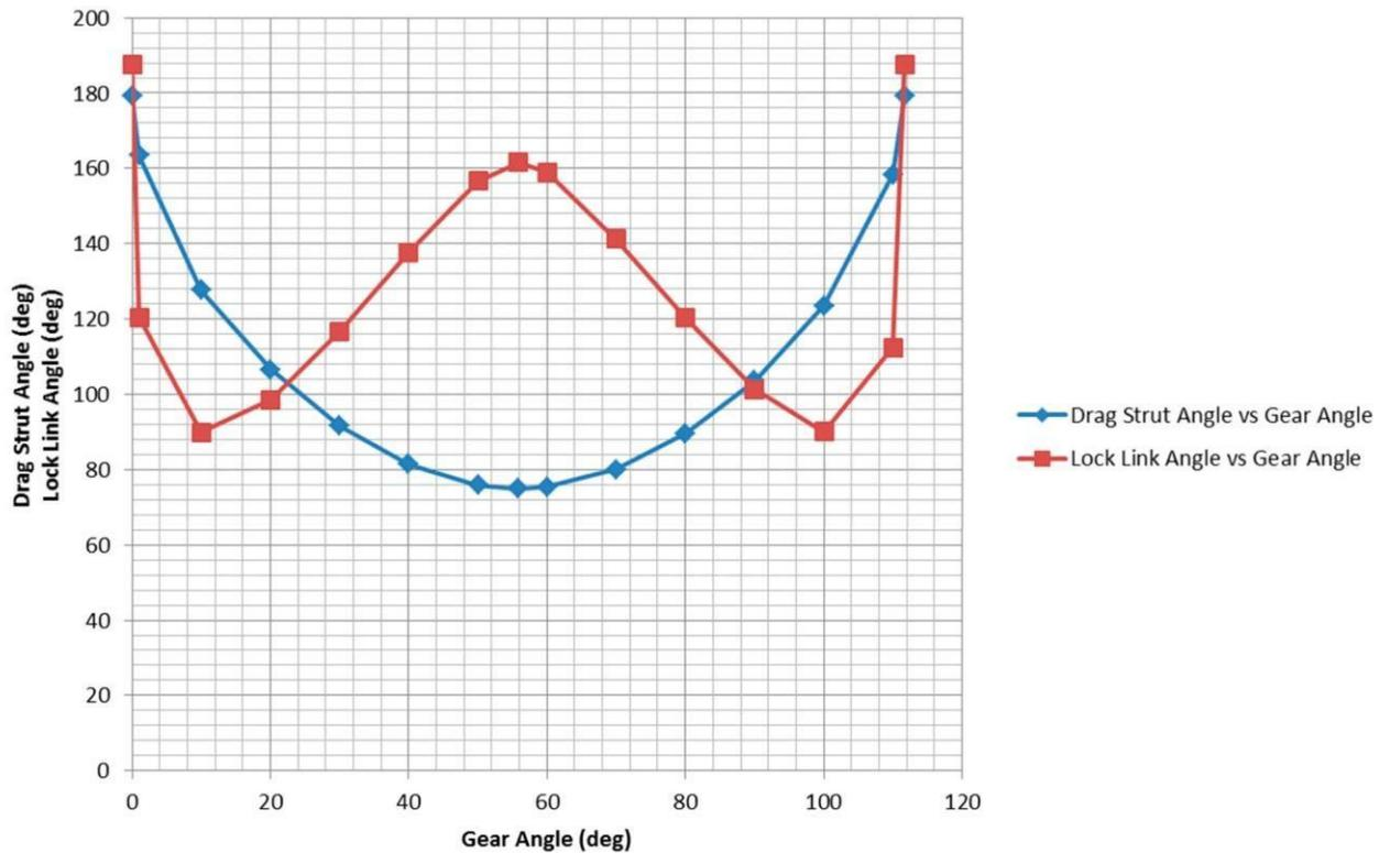
**Picture 77 Drag Strut Angle and Lock Link Angle vs Gear Angle**
