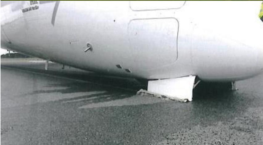
**Picture 16 and 16A** After the aircraft had come to a complete stop on the runway the NLG appeared to have fully collapsed, which resulted in NLG front door damage.
