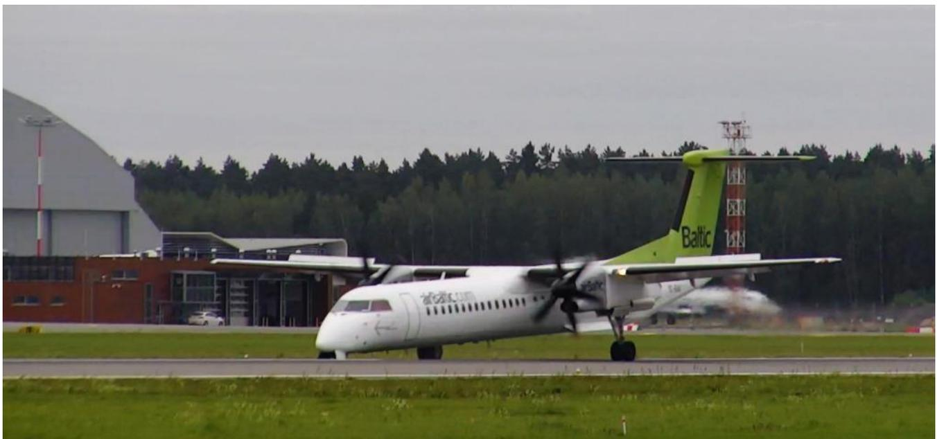
**Picture 15** After landing the NLG collapsed but not abruptly but progressively, because NLG doors didn't touch RWY surface right away after touching.
