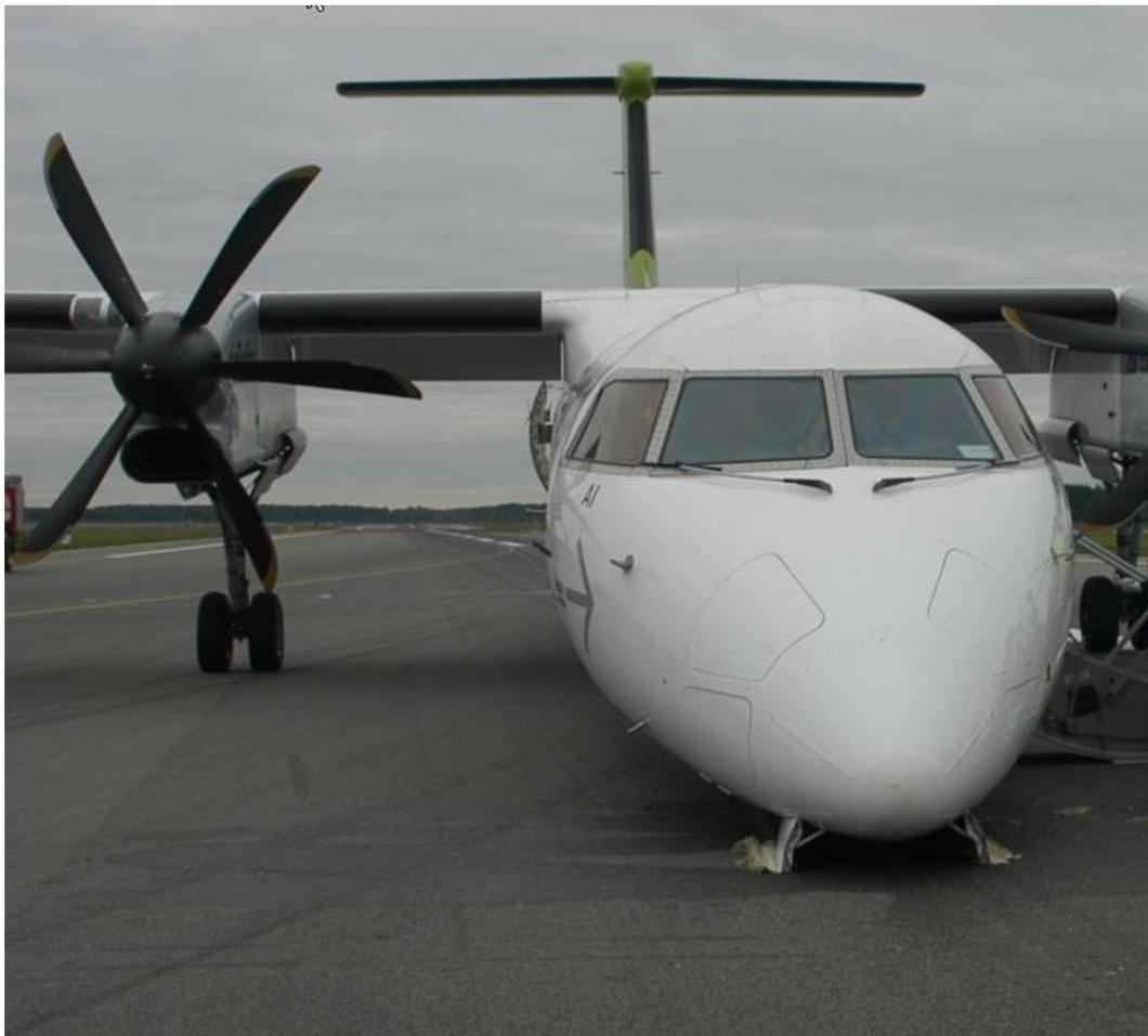
**Picture 23 NLG front doors damage**
