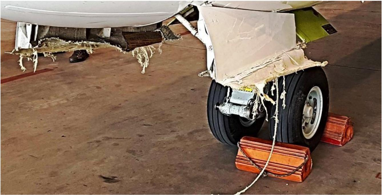
**Picture 17 Damages of NLG front doors**
