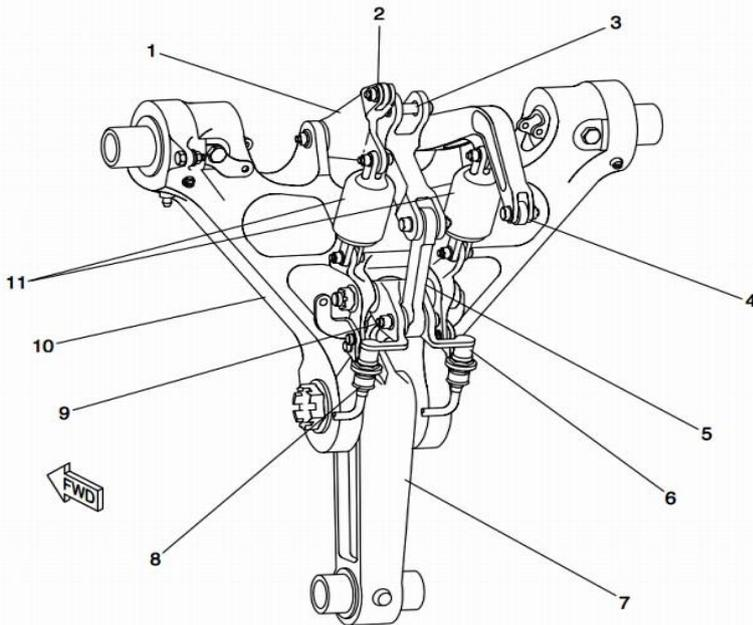
The drag strut assembly stabilizes the shock strut in either the retracted or the extended position. The drag strut assembly has the components that follow:
