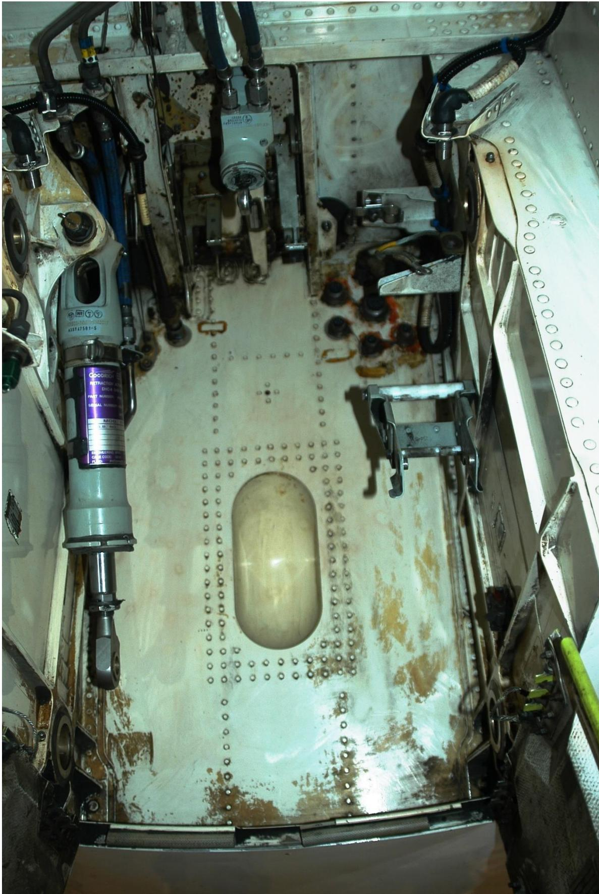
**Picture 30 NLG compartment after components removing.**
