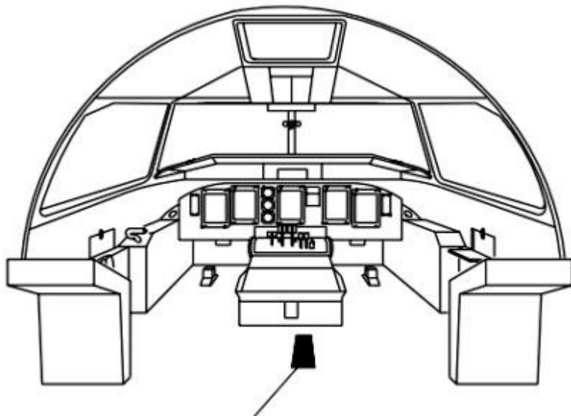
**NLG alternate release locator**
