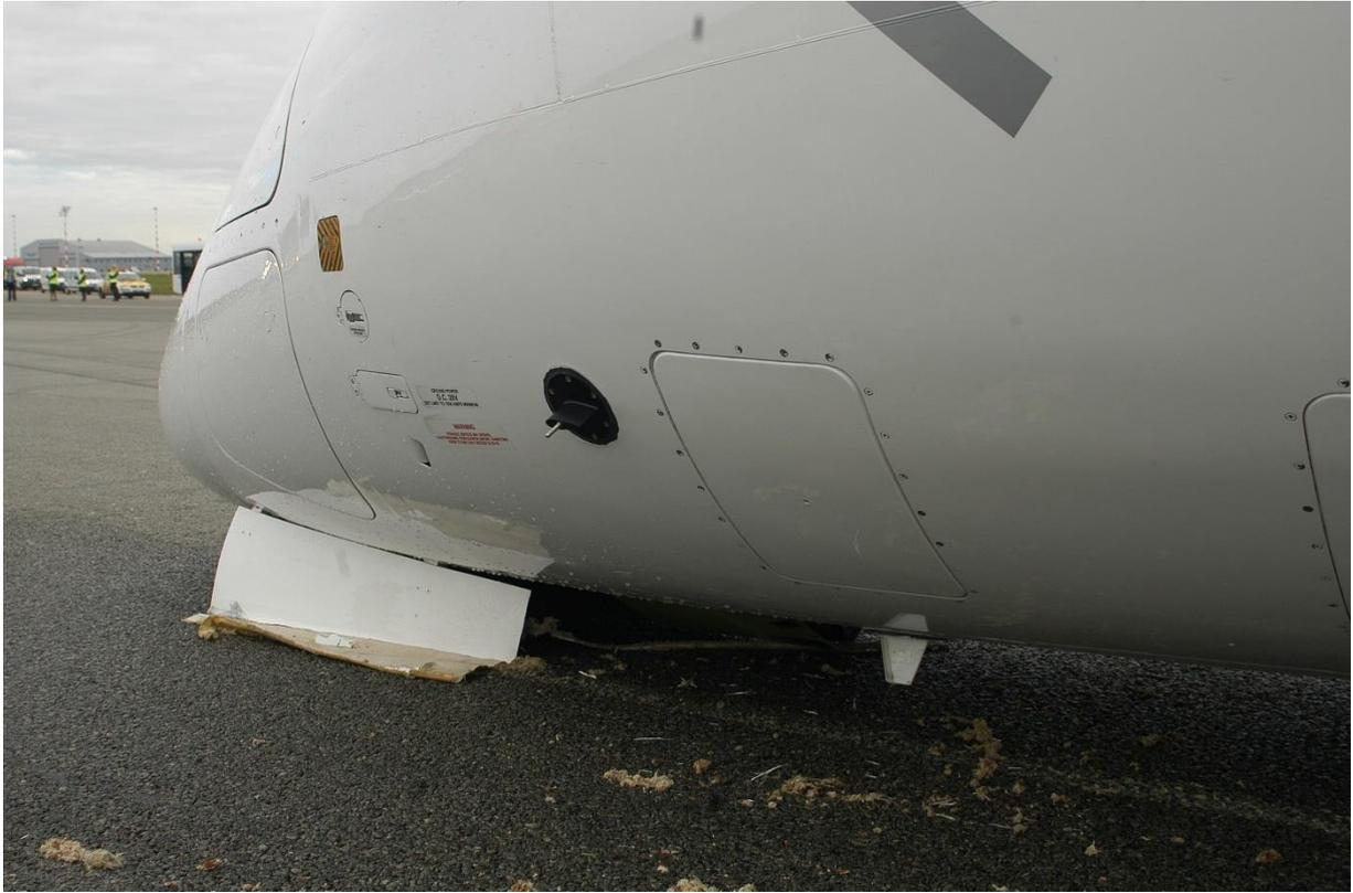
**Picture22 NLG front doors damage**
