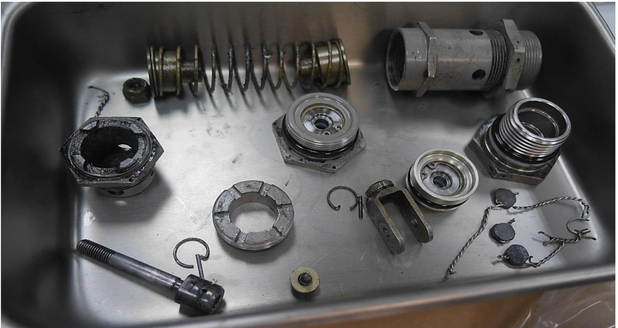
Photo 38: Centering spring assembly, and other parts associated with the spool and sleeve assembly
