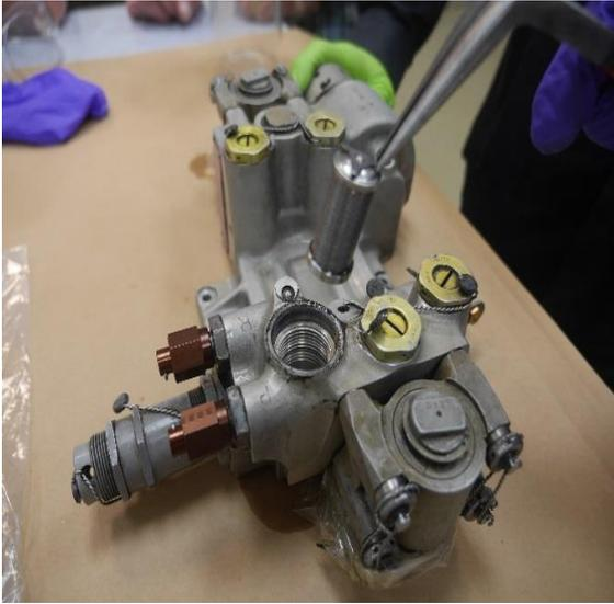
Photo 35: Filter being removed from steering metering valve
