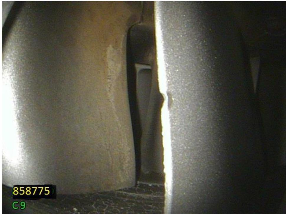
Photo 9: HPC ST9 surface damage
