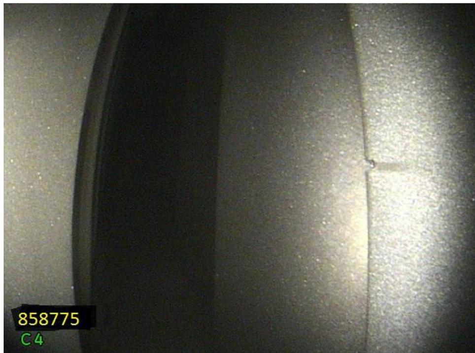
Photo 8: HPC ST4 surface damage
