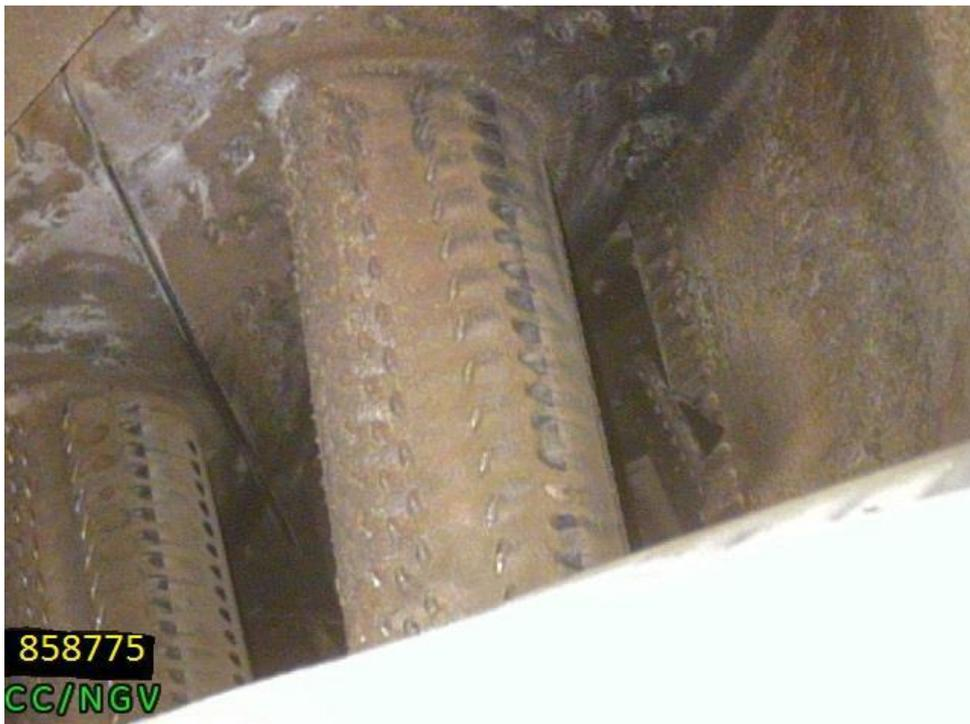
Photo 10: Dirt on the Nozzle Guide Vanes
