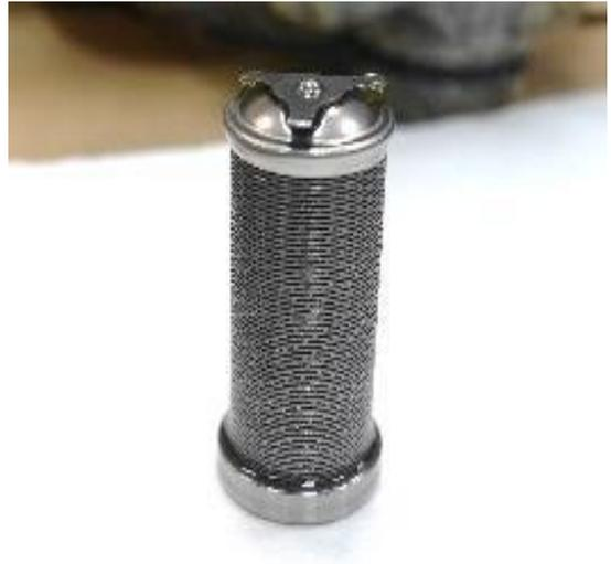
Photo 36: Filter removed from steering metering valve
