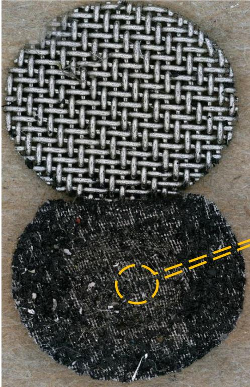
Photo 40a: Bleeder filter separated in two
