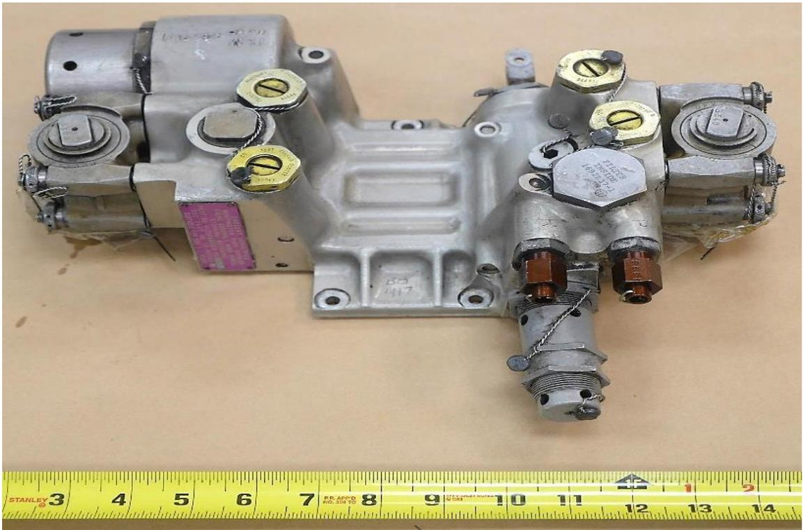
Photo 32: Overview of steering metering valve
