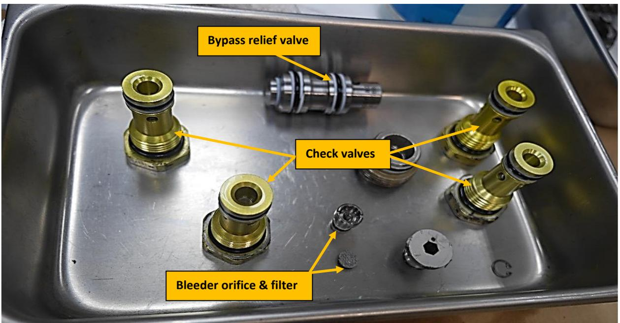
Photo 39: Valves and bleeder orifice removed from steering metering valve
