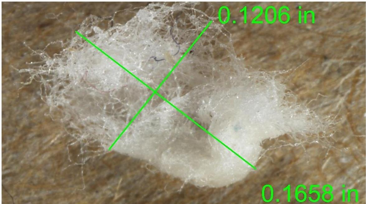
Photo 37: Detailed view of fibrous debris with measurements
