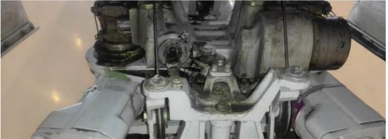
Photo 30: The nose gear steering metering valve before disassembly
