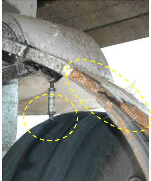
Photo 2: L/H Main gear Inner door with broken Inner pushrod
