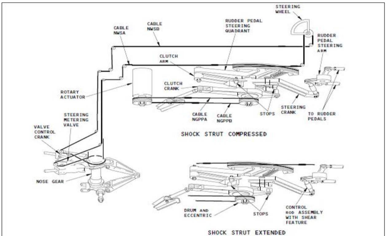
Scheme 2: Nose wheel steering Schematic
