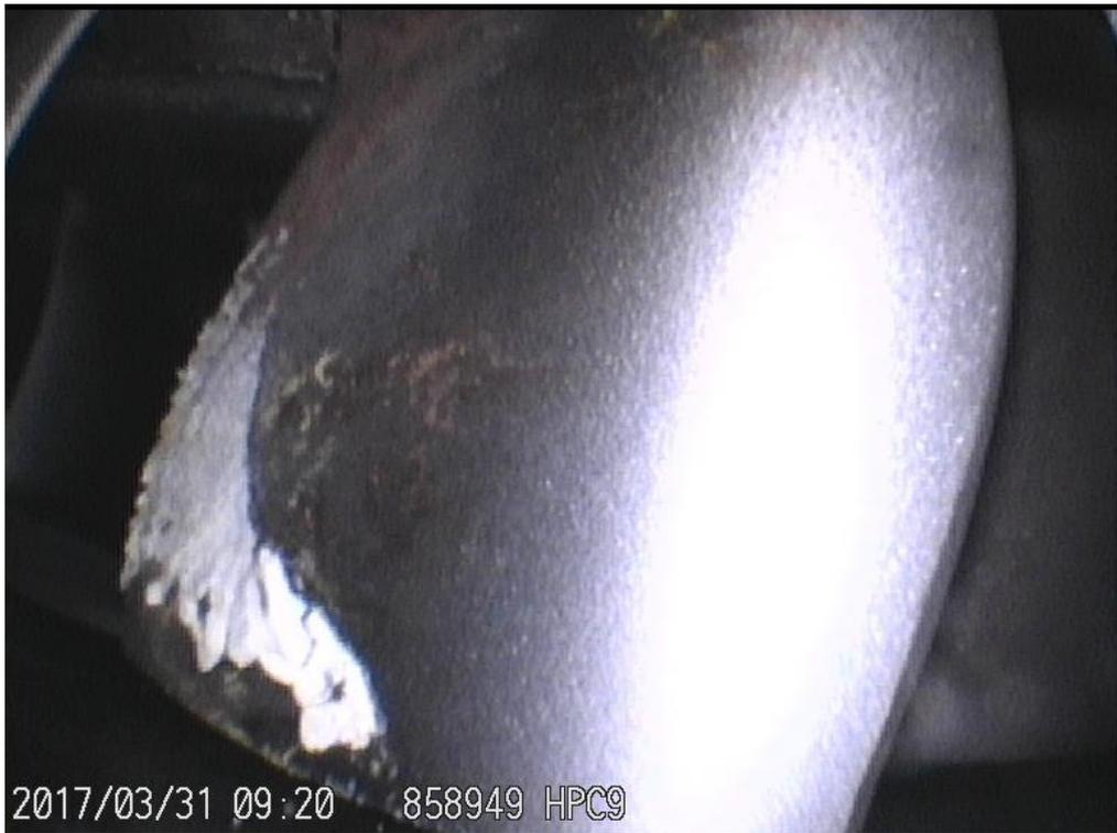
Photo 15: Corrosion marks on the HPC ST9
