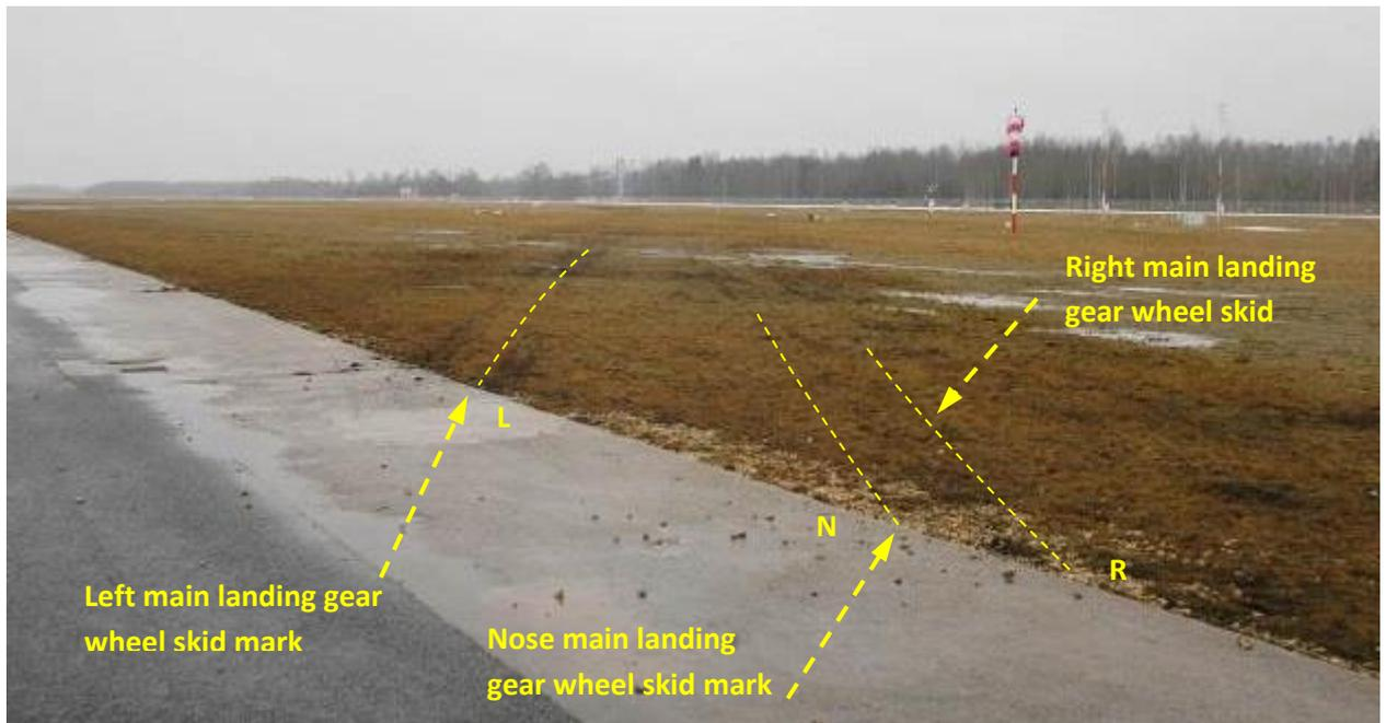
Photo 41, Aircraft takeoff roll trajectory
