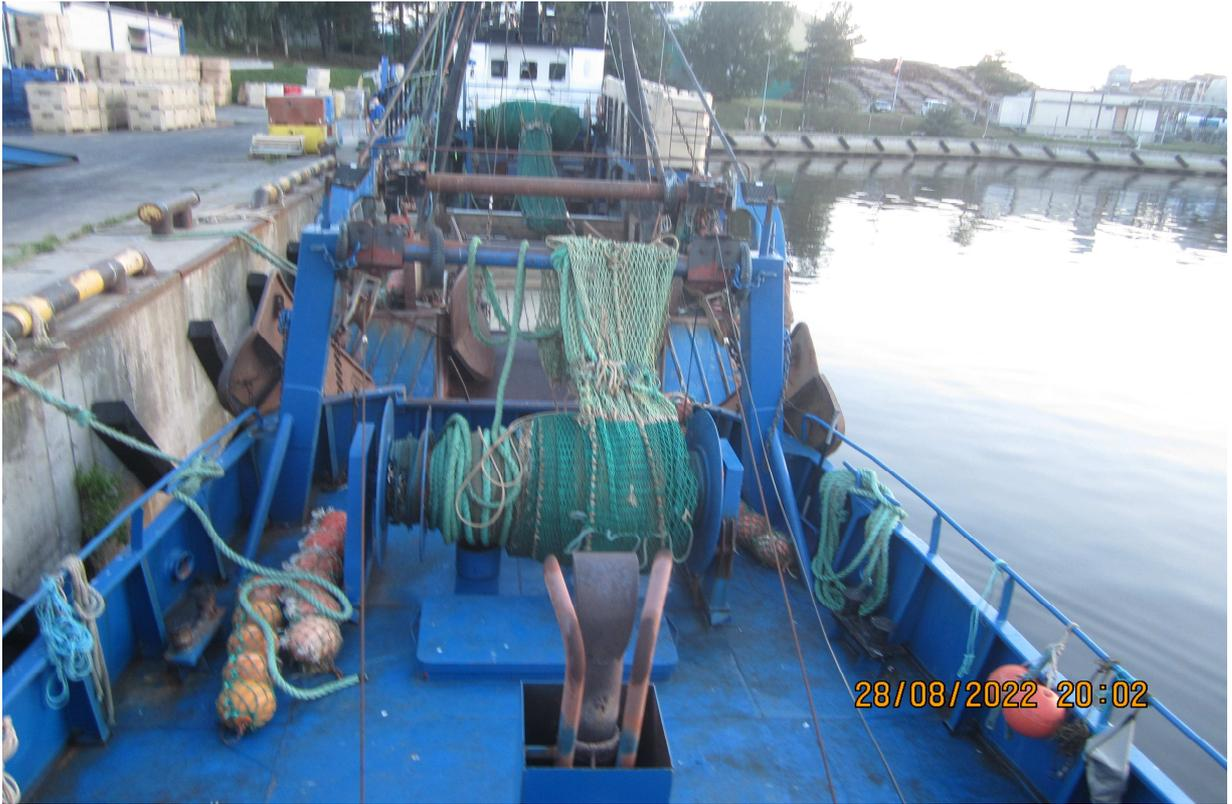
Figure 3. Trawl winch
