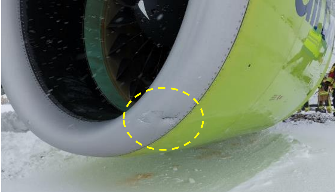
Picture 7: Damage of the Inlet Cowl of the LH Engine
