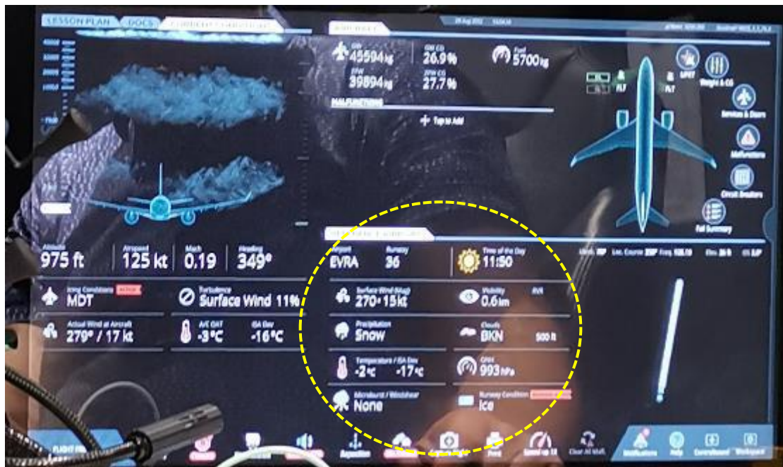
Picture 22: Setting of maximum data in the simulator for landing
