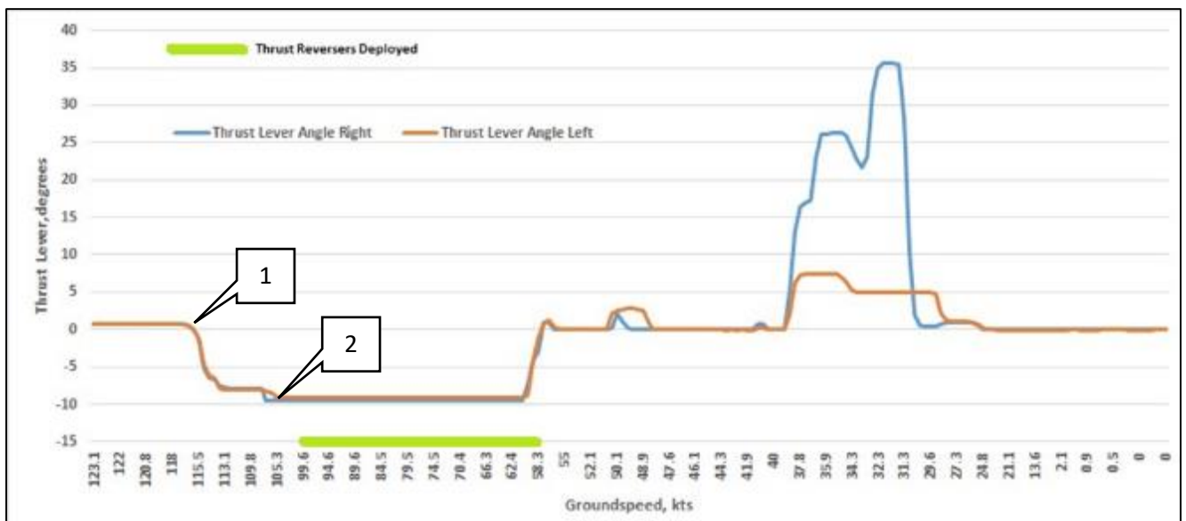
Picture 13: Fragment from FDR data plots of thrust levers
