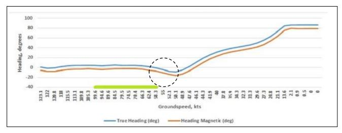
Picture 12: Fragment from FDR data plots of the aircraft heading
