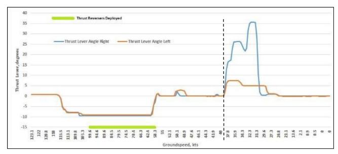
Picture 17: Fragment from FDR data plots of thrust levers
