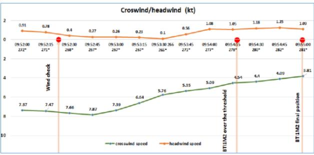
Picture 4: Crosswind/headwind during landing of the RIX
