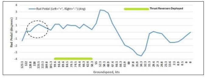
Picture 11: Fragment from FDR data plots of rudder pedal
