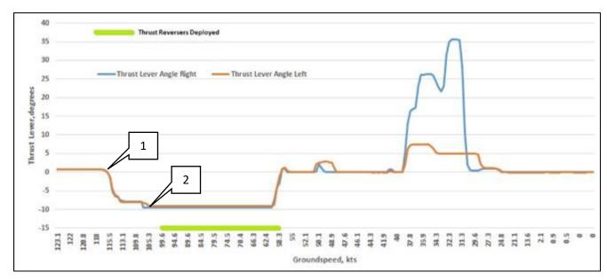
Picture 13: Fragment from FDR data plots of thrust levers
