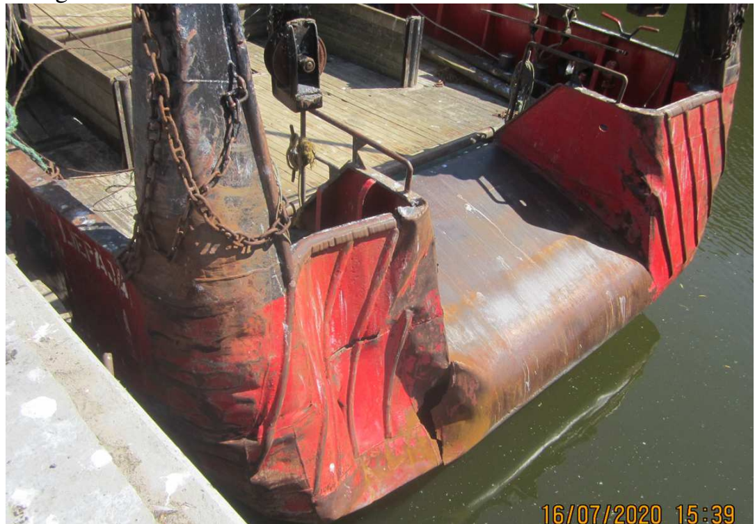
Image 4: Damaged part of MARITA on her aft
