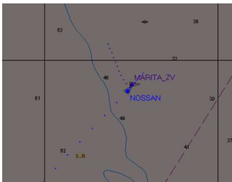
Image 3: AIS playback’s snapshot of collision moment. MARITA’s trajectory exposes avoidance manoeuvre 1-3 minutes before collision.
