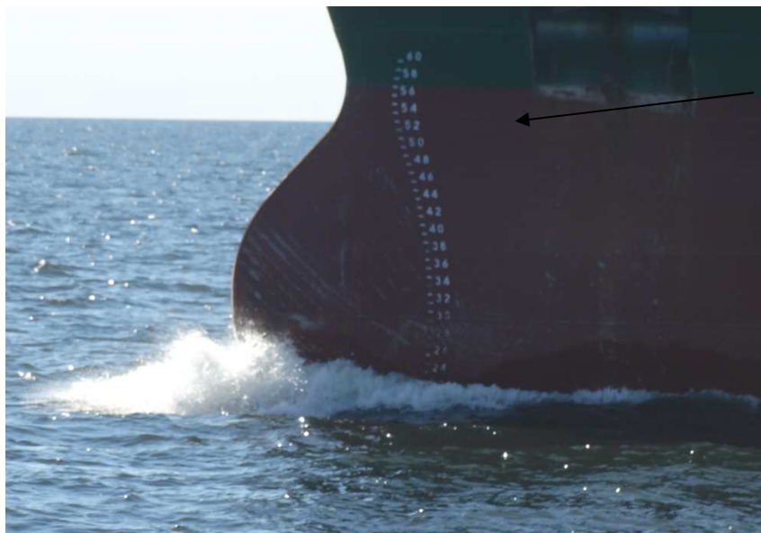
Image 5: NOSSAN' bulb with visible scratches on. Photo has taken by Coast Guard shortly after collision with MARITA
