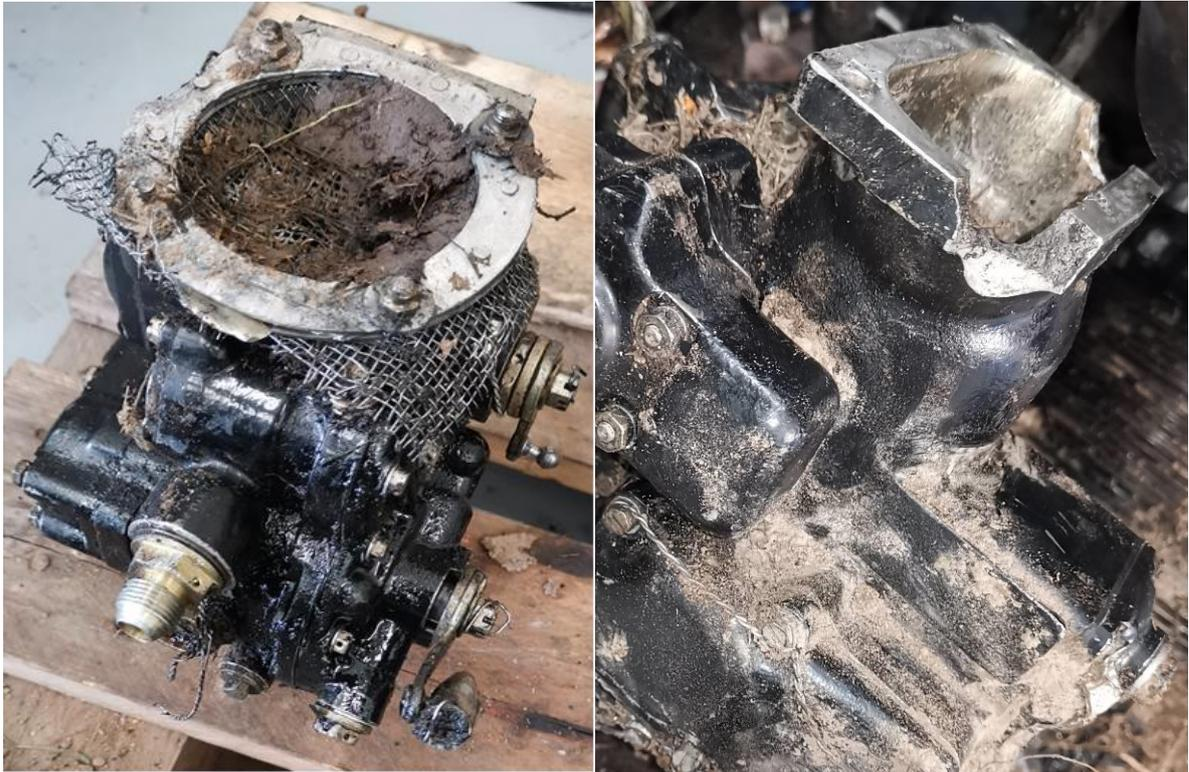
Picture 22: The engine carburettor
