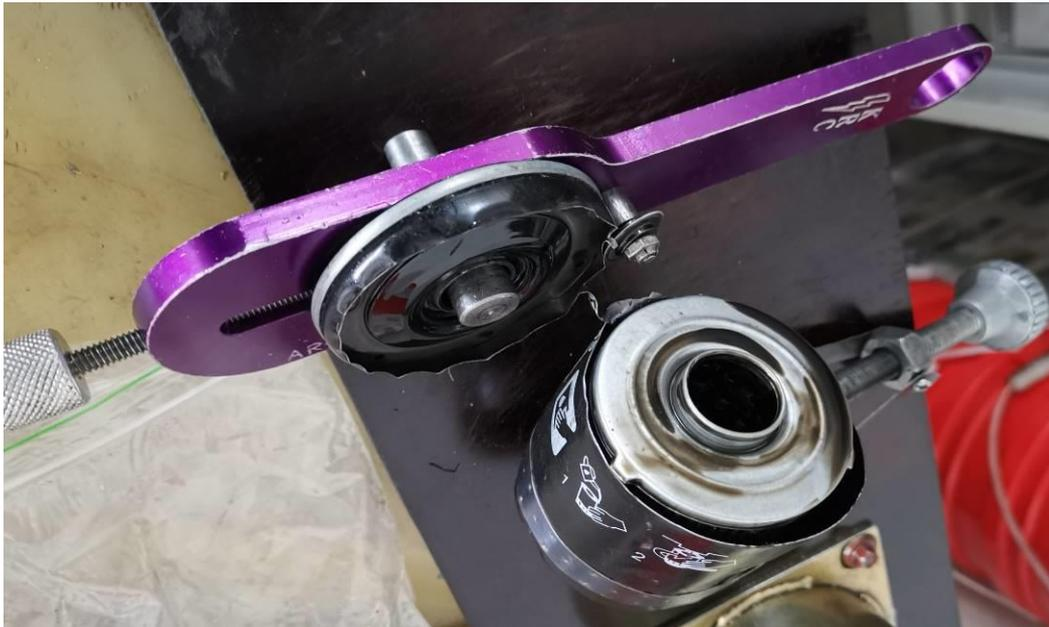
Picture 24: Opened oil filter housing
