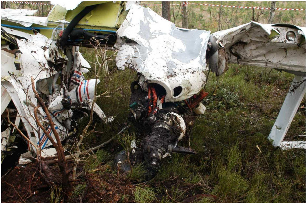
Image19. Left side engine after pulling out of the ground
