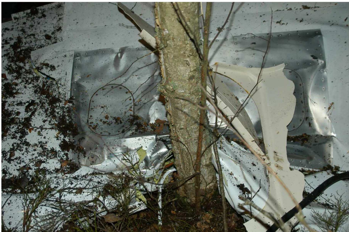
Image6. The right wing has been deformed due to the impact, colliding with the tree stem;
