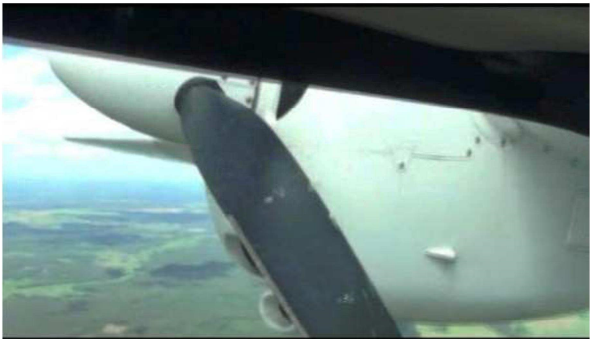
Image25. Propeller of the right side engine does not rotate
