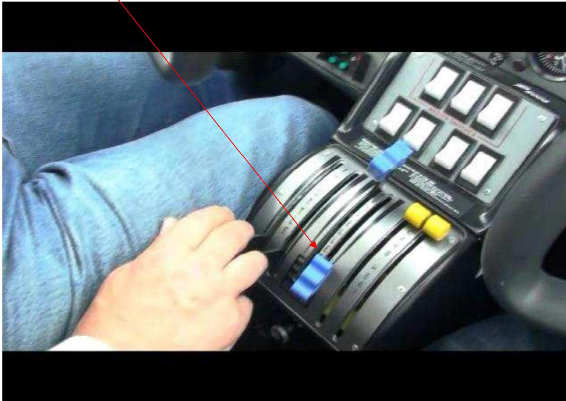
Image 26. Right side engine propeller has been locked, the throttle of the operating engine – partly closed
