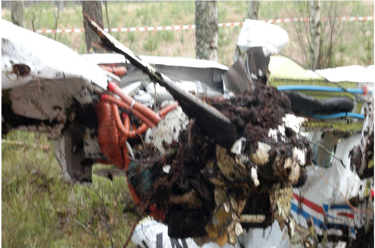
Image17. Right side engine after pulling out of the ground Propeller blade of the right side engine was in position parallel to the airflow (propeller feathered)
