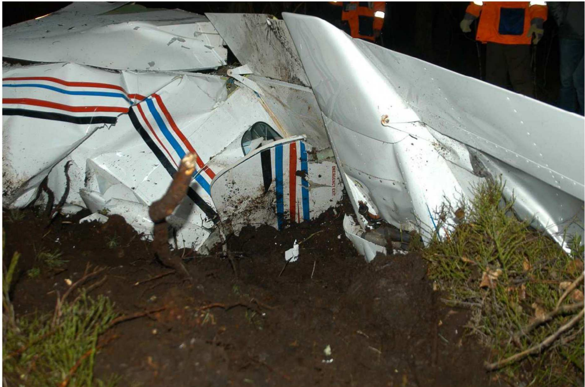
Image7.Tail of the aircraft fuselage (rudder, fin and vertical stabiliser) is broken off from fuselage.
