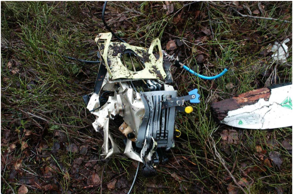
Image10. Handles of the controlling device „Central Pedestal” body are deformed and broken
