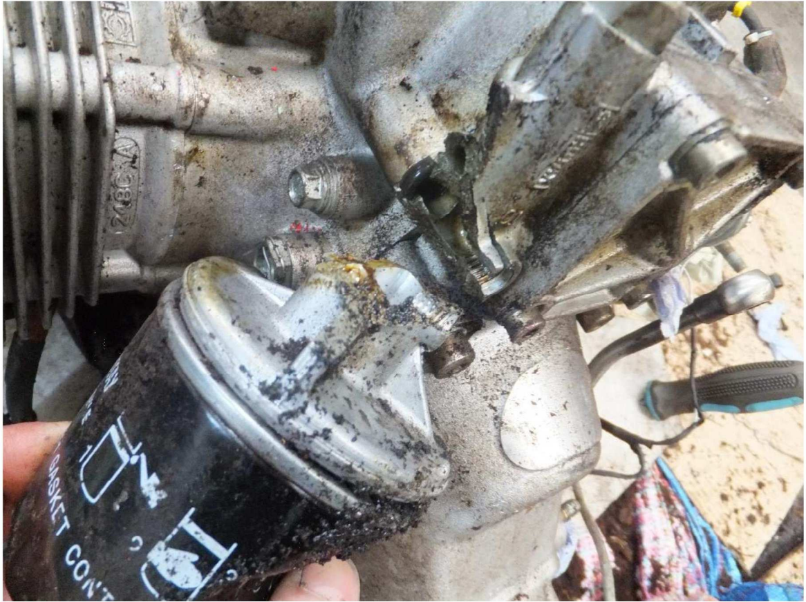
Image 30. Oil filter fastening flange at oil pump is broken
