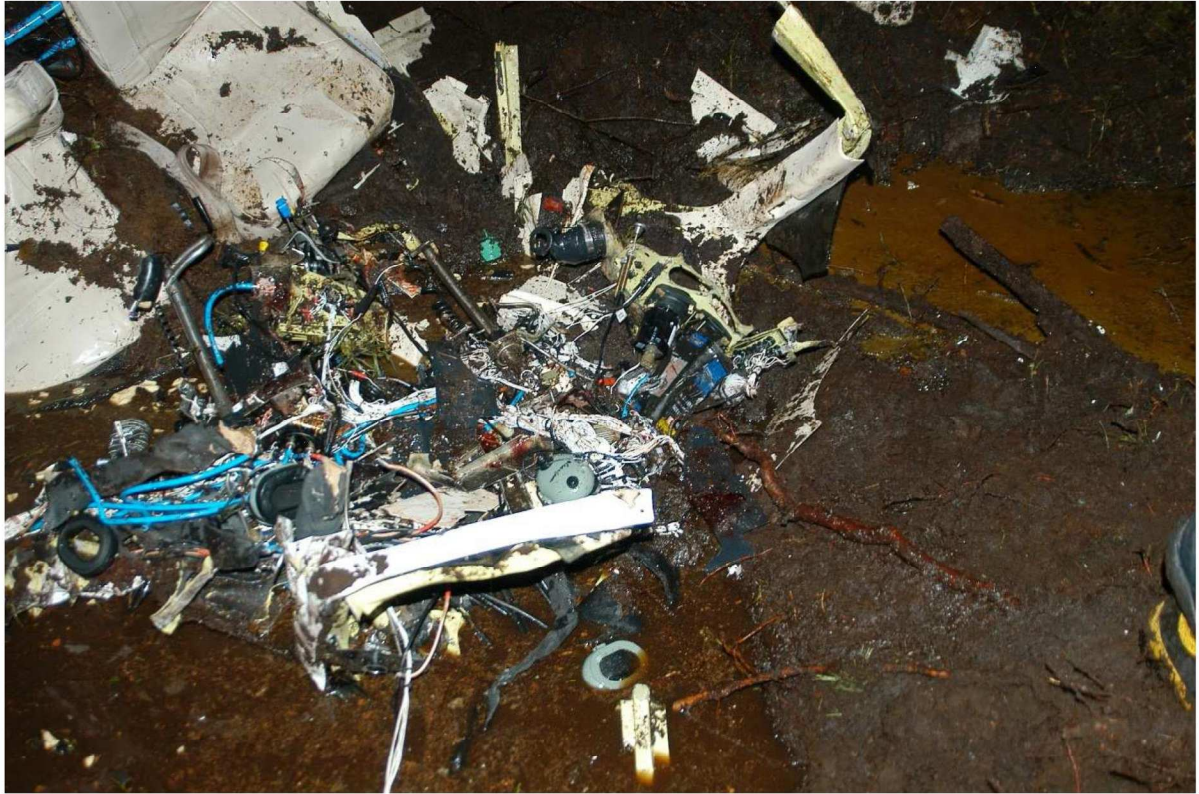
Image9. Forepart of the aircraft including instrument panel is fully destroyed.
