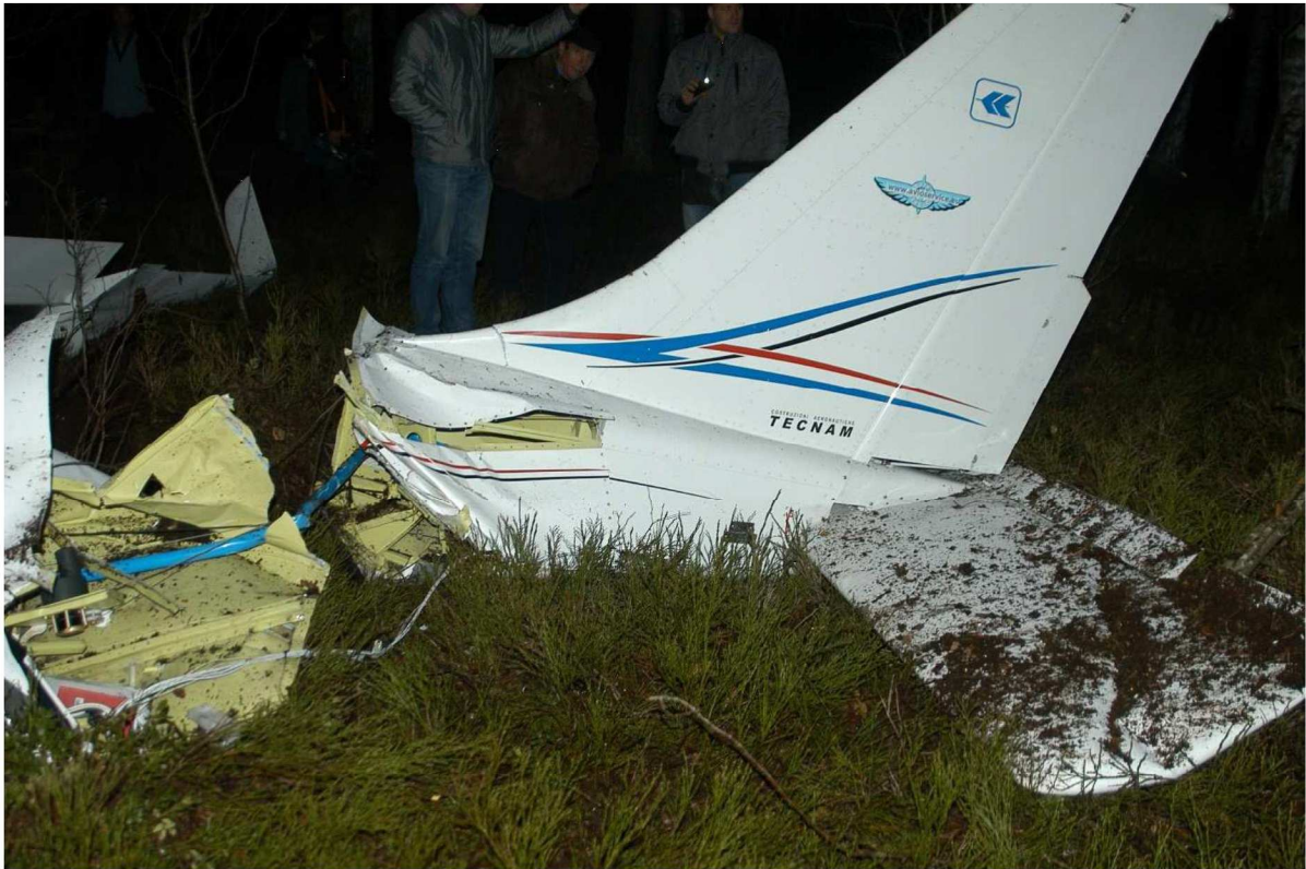
Image7.Tail of the aircraft fuselage (rudder, fin and vertical stabiliser) is broken off from fuselage.
