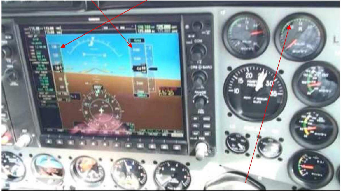
Image24. Propeller rotation of the right side engine (rpm)
