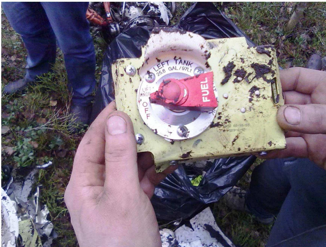
Image18. On the Right hand Fuel selector, found at the accident site, valve was in the position "OFF"
