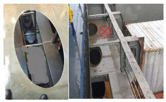
Fig. 2. Left: Lightening hole in guide cell area of the ship; Right: twin deck within cell area; assumed standing point of stevedore (between guardrail and opening) before the accident is marked by red symbol.
