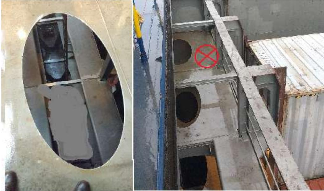
Fig. 2. Left: Lightning hole in guide cell area of the ship; Right: twin deck within cell area; assumed standing point of stevedore (between guardrail and opening) before the accident is marked by red symbol.
