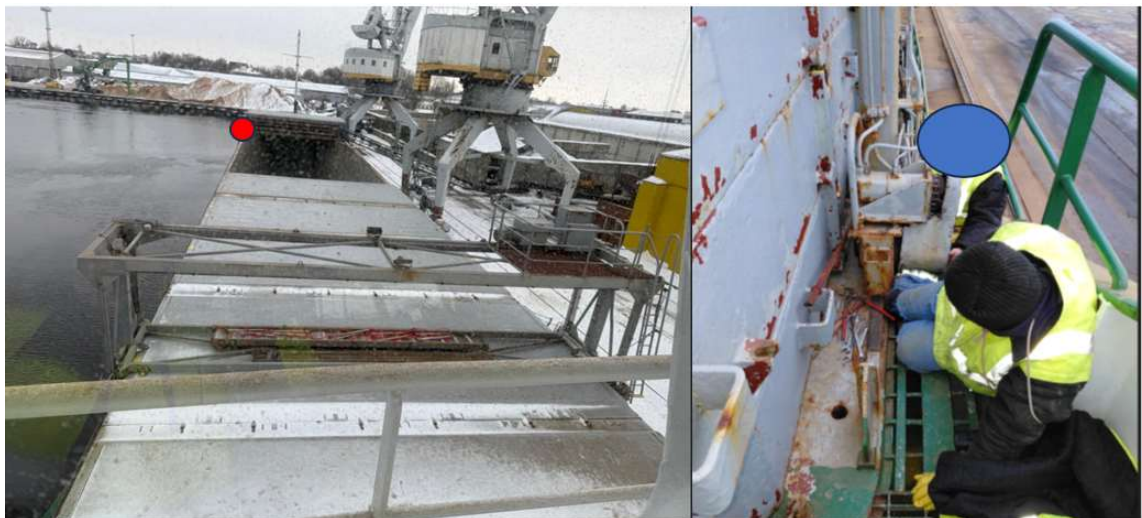
Image 3. Location onboard (by red dot, view from bridge) and visualisation of trapped leg at moving part of gantry crane at vessel's fore deck
