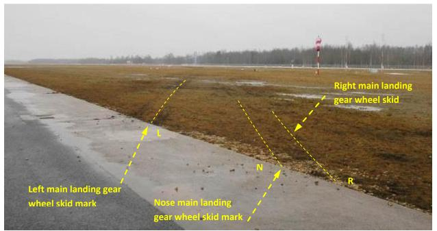
Photo 41, Aircraft takeoff roll trajectory
