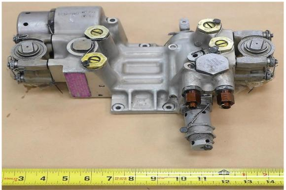
Photo 32: Overview of steering metering valve
