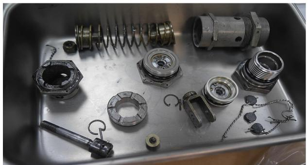
Photo 38: Centering spring assembly, and other parts associated with the spool and sleeve assembly
