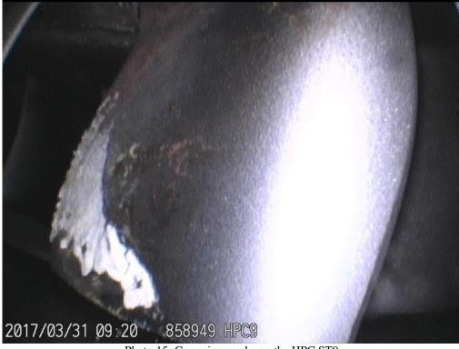
Photo 15: Corrosion marks on the HPC ST9
