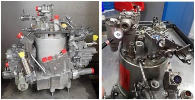
Photo 22a/b: The MEC equipment visual check
