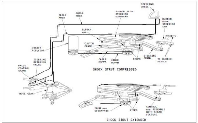
Scheme 2: Nose wheel steering Schematic
