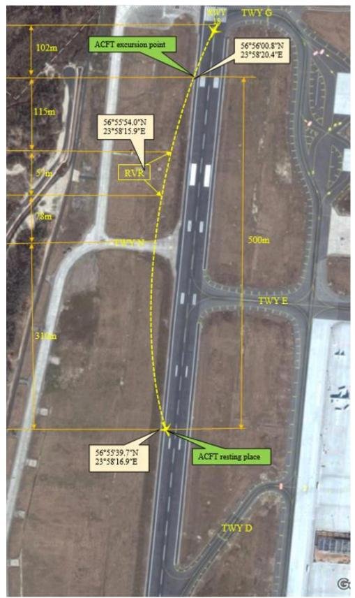
Scheme 1 the aircraft Boeing 737-524, VP-BVS movement's scheme on the RWY 18
