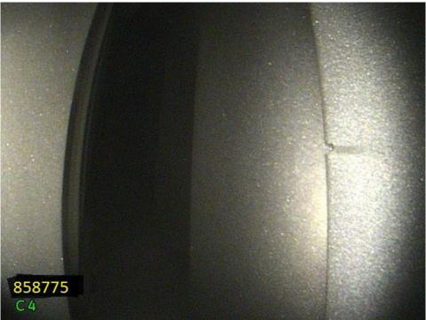
Photo 8: HPC ST4 surface damage
