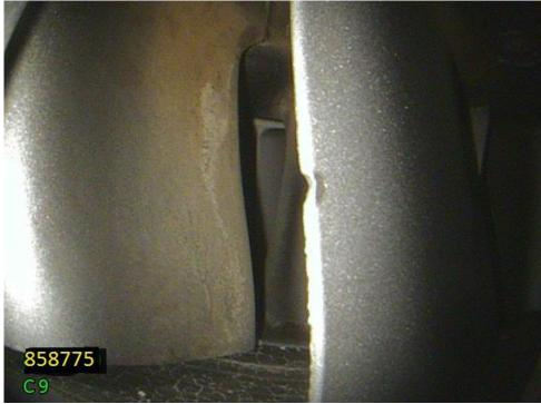
Photo 9: HPC ST9 surface damage
