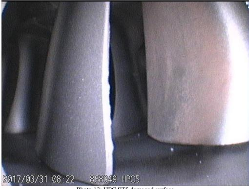
Photo 13: HPC ST5 damaged surface
