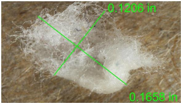
Photo 37: Detailed view of fibrous debris with measurements
