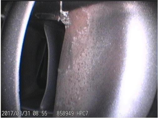
Photo 14: Corrosion marks on the HPC ST7
