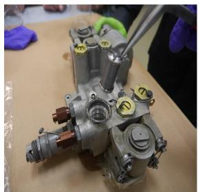
Photo 35: Filter being removed from steering metering valve
