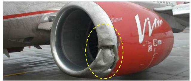
Photo 3: L/H Engine Inlet Cowl Inner and Outer, Overboard Fan Cowl Panel
