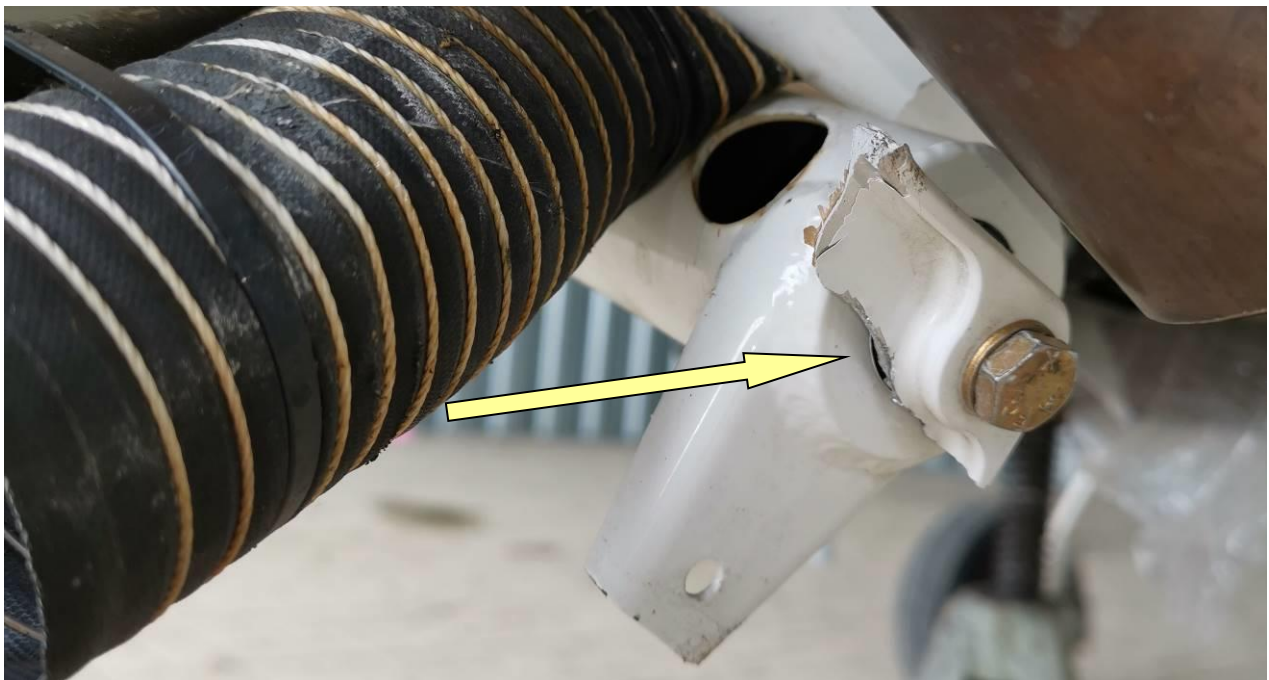
Figure 4. Breaking point of the left-side angle flange of the nose landing gear leg
