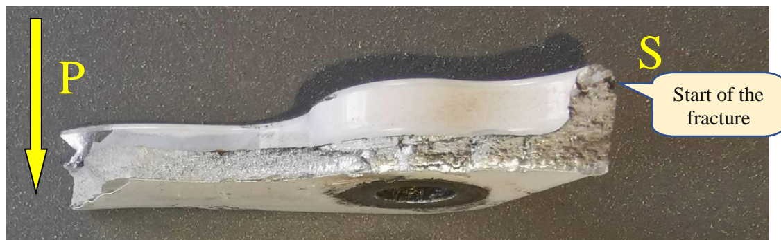
Figure 14. Image of the fracture surface of the part that has broken off
