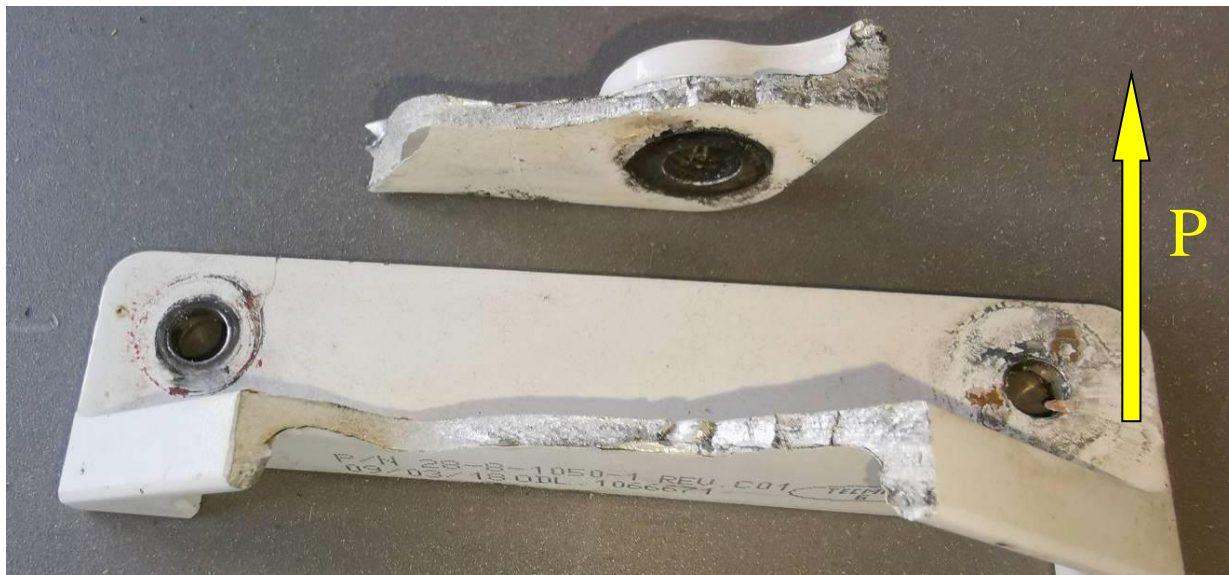
Figure 11. Both fractured parts of the left-hand flange and the action direction of force P
