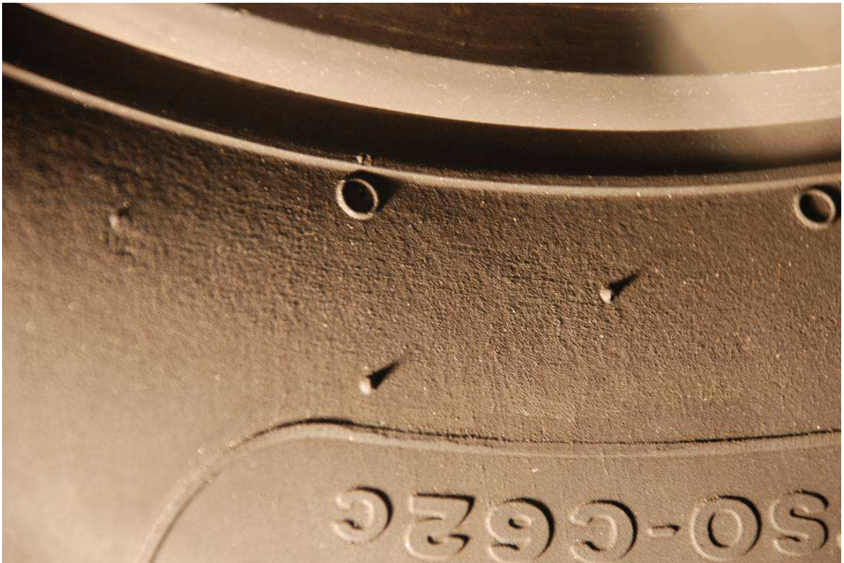
Figure 9. Tire sidewall surface evidence of fire, detail
