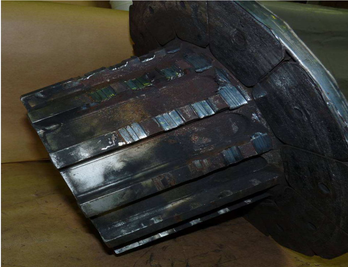
Figure 39. Torque tube assembly spline damage
