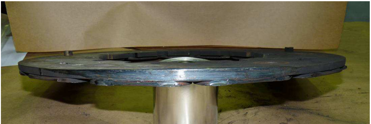
Figure 34. Pressure plate rotational damage
