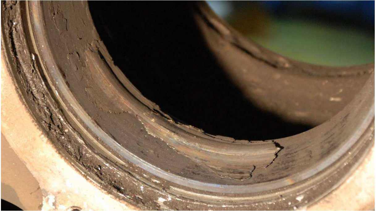
Figure 14. Hub with bearing cup of outboard wheel half, detail
