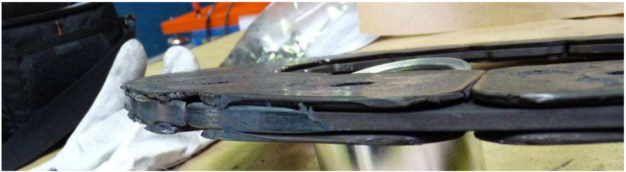
Figure 35. Damage to the lower segment of stator disk
