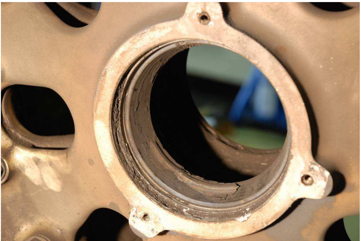
Figure 13. Hub with bearing cup of outboard wheel half
