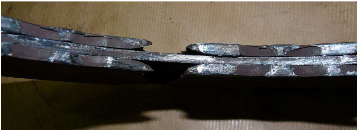
Figure 38. Damage to inner circumference of rotor disk
