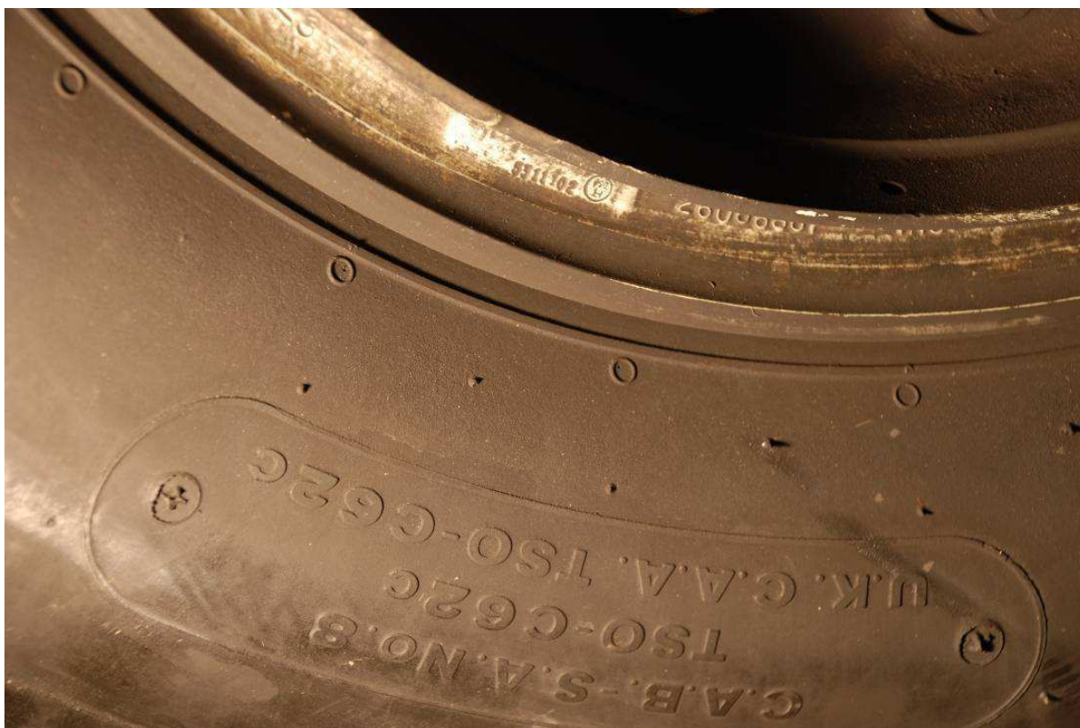
Figure 8. Tire sidewall surface, evidence of fire
