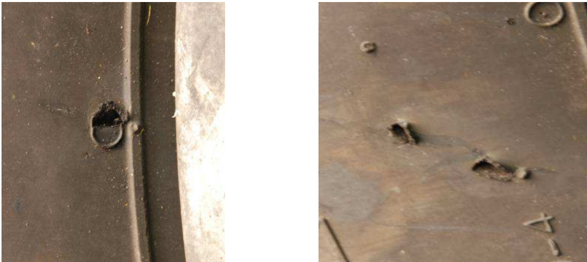
Figure 12. Cuts in tire sidewall
