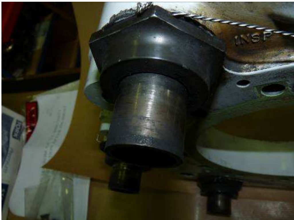
Figure 32. Piston with fire damage
