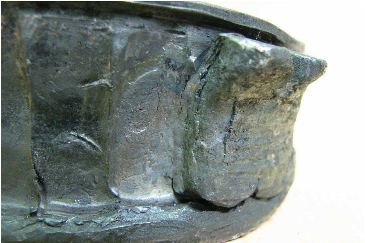
Figure 22. Outboard bearing inner race, crushed rollers (3)
