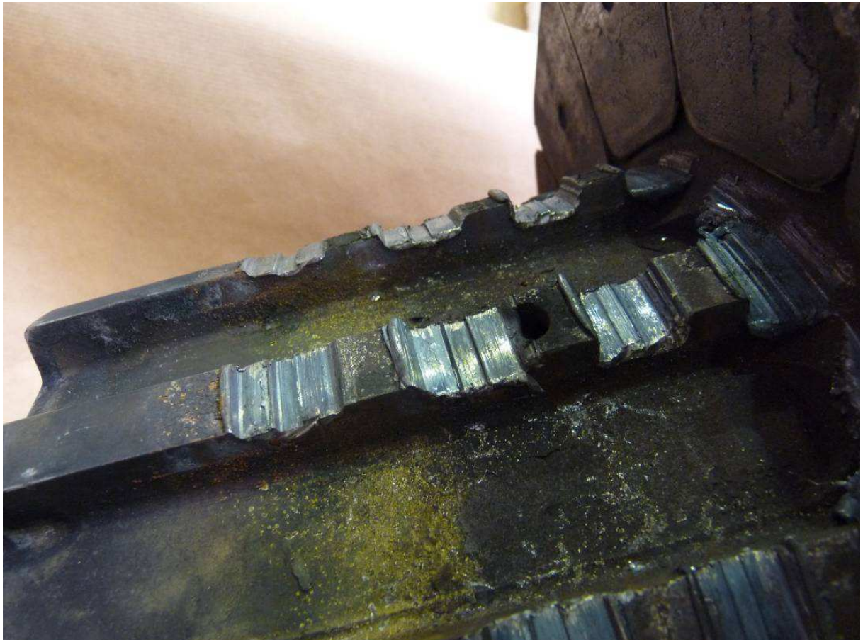
Figure 40. Difference in indentation caused BYR stuck rotor segment
