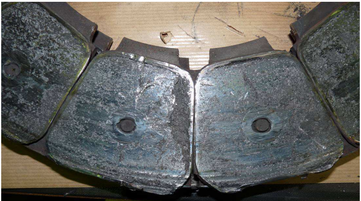
Figure 36. Brake lining crumbling and creep
