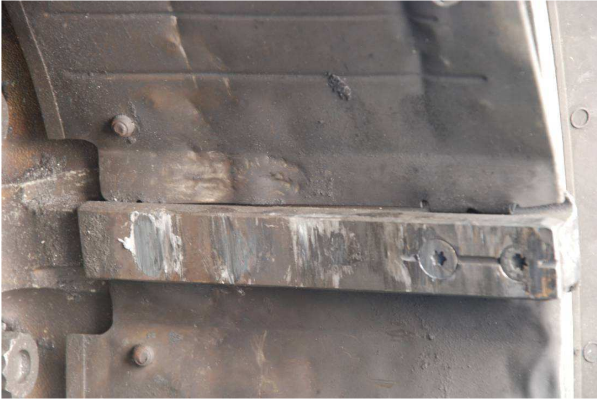
Figure 17. Damage to heat shield and rotor drive keys
