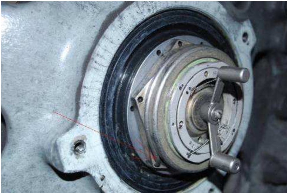
Figure 5. To prevent nut coming loose during operation nut is locked with AXLE NUT RETAINER RING, which locks WASHER and nut together
