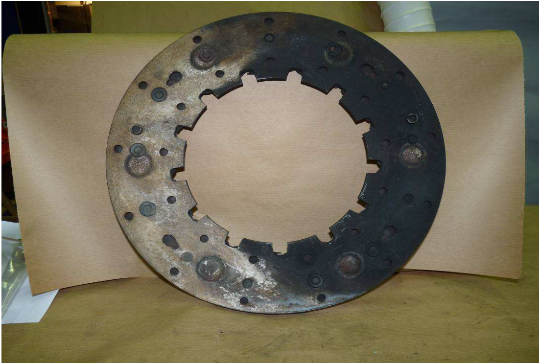
Figure 33. Pressure plate fire damage
