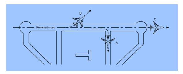
Picture 13. Position limits to be reached by a landing aircraft A or a departing aircraft B or C before an arriving aircraft may be cleared to cross the threshold of the RWY or a departing aircraft may be cleared to take off
