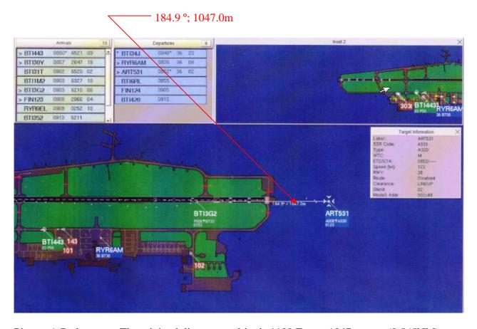
Picture 6. Radar map - The minimal distance at altitude 1100 Ft was 1047 meters (0.565NM)
