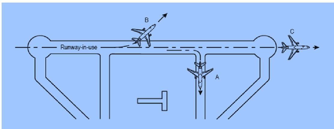
Picture 13. Position limits to be reached by a landing aircraft A or a departing aircraft B or C before an arriving aircraft may be cleared to cross the threshold of the RWY or a departing aircraft may be cleared to take off
