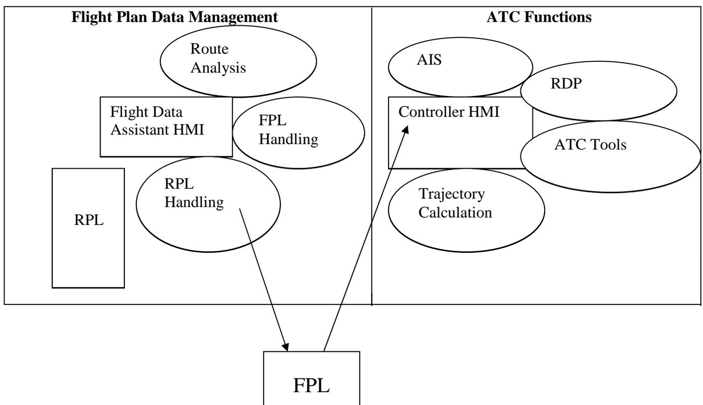
The distinct border is between the Flight Plan Data Management block and the ATC Functional block.
