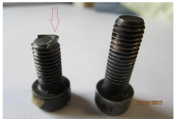
Fig.19 Fractured screw and missing one
