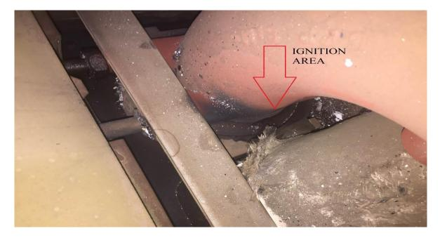
Fig.16.Exhaust from cylinder A6, ignition of Fuel Oil
