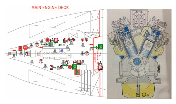
Fig.2 ME Deck layout showing fire zones
