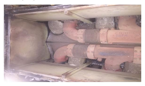
Fig.15 Exhaust manifold on the top of the engine
