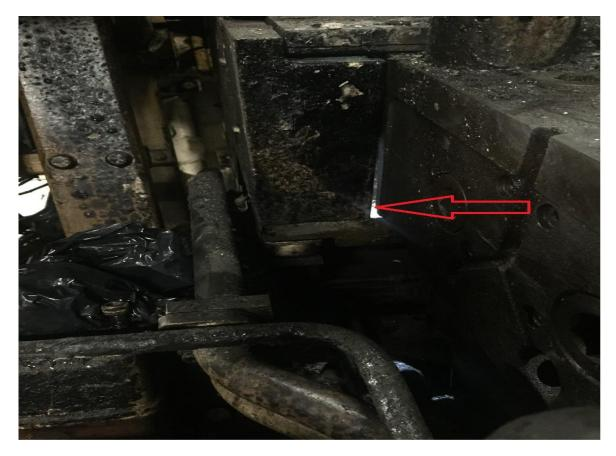
Fig.14 Arrow shows the gap in insulation of manifold cover, illuminated from inside.
