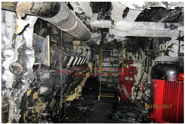
Fig.13 ME Deck Port side forward end, arrow shows where the fire started
