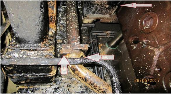
Fig.17: arrow 1-fractured screw, arrow 2-missing screw, arrow 3-gap in manifolds insulation box.
