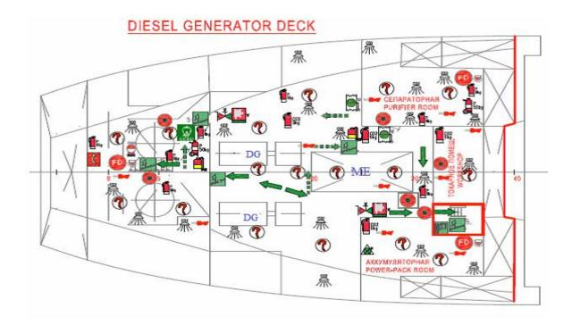
Fig.5 DG Deck layout showing fire zones
