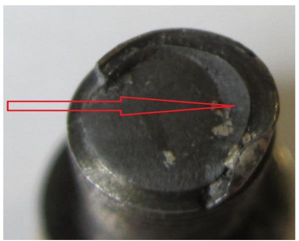
Fig.20 Area where fatique developed under banding loads.
