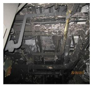
Fig.9 ceiling of engine room
